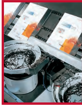
Double automatic hanger feeder.
