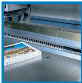
The wire in the tool ready for binding.
